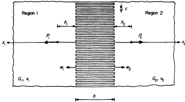
Fig. 1. Geometry and loading of the composite plate [suffixes 1 and 2 refer to the halfplane regions 1 and 2 respectively].
