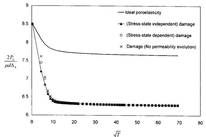
**Fig. 8.** Numerical results for transient translational displacement of rigid rock socket ( $L/d=1.0$ ) embedded in brittle poroelastic half space (impervious interface)
