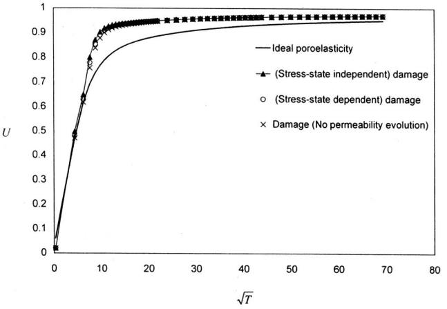
**Fig. 10.** Numerical results for degree of consolidation for rigid rock socket ( $L/d=1.0$ ) embedded in brittle poroelastic half space (pervious interface)
