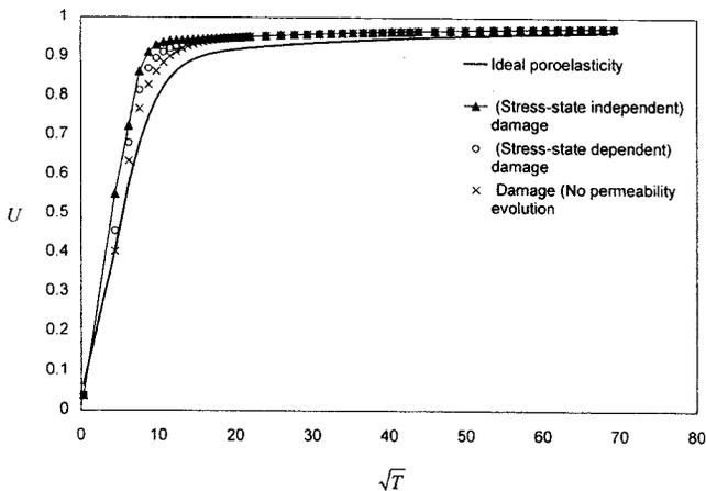
**Fig. 15.** Numerical results for degree of consolidation for rigid rock socket ( $L/d=2.0$ ) embedded in brittle poroelastic half space (pervious interface)
