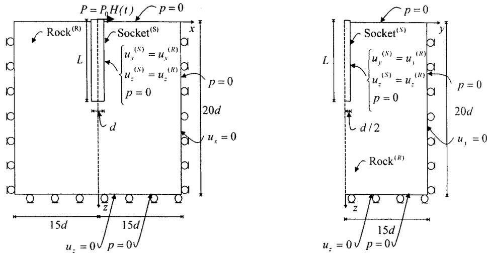
**Fig. 4.** Boundary conditions for pervious interface between rock socket and geomaterial
