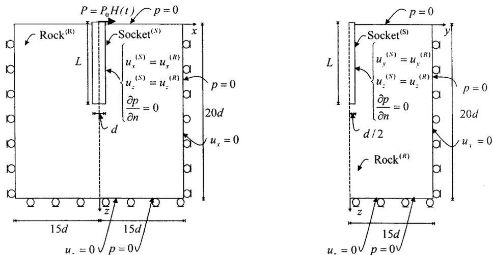
**Fig. 5.** Boundary conditions for impervious interface between rock socket and geomaterial
