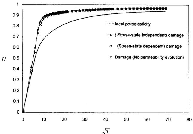
**Fig. 11.** Numerical results for degree of consolidation for rigid rock socket ( $L/d=1.0$ ) embedded in brittle poroelastic half space (impervious interface)
