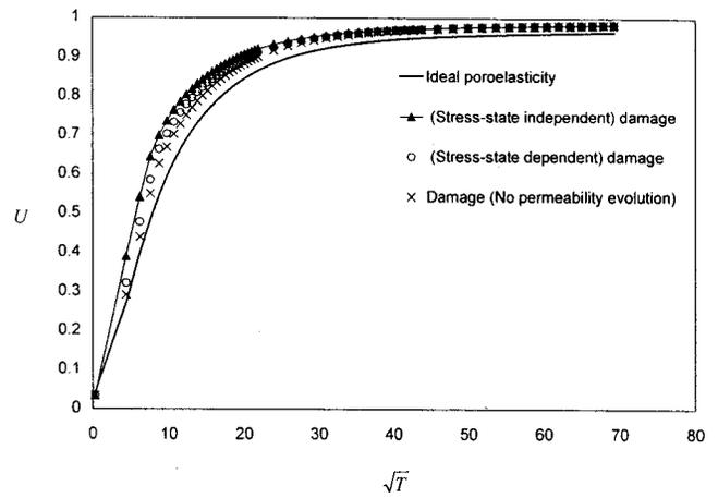
**Fig. 21.** Numerical results for degree of consolidation for rigid rock socket ( $L/d=4.0$ ) embedded in brittle poroelastic half space (impervious interface)
