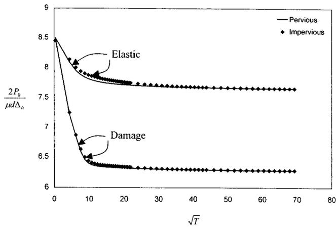
**Fig. 9.** Comparison of results for rigid rock socket with ( $L/d=1.0$ ) with either pervious or impervious interface between rock socket and poroelastic half space.
