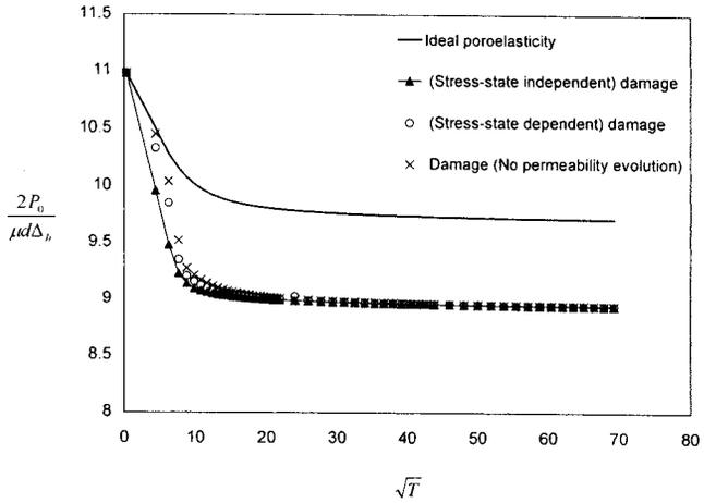
**Fig. 12.** Numerical results for transient translational displacement of rigid rock socket ( $L/d=2.0$ ) embedded in brittle poroelastic half space (pervious interface)
