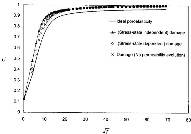
**Fig. 20.** Numerical results for degree of consolidation for rigid rock socket ( $L/d=4.0$ ) embedded in brittle poroelastic half space (pervious interface)
