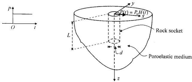
**Fig. 1.** Laterally loaded rigid rock socket embedded in poroelastic geomaterial
