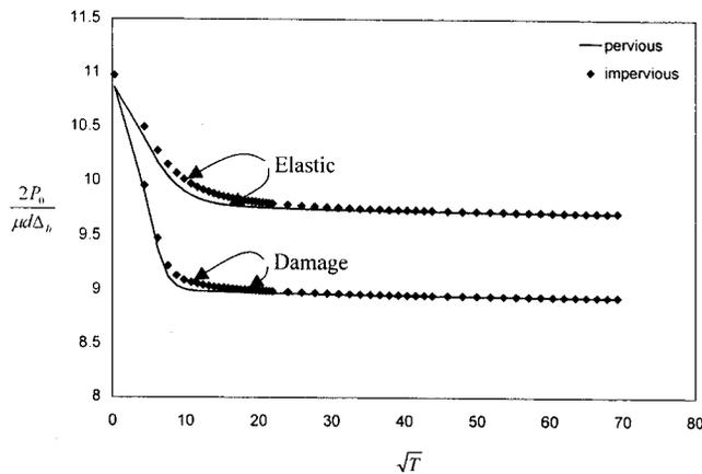
**Fig. 14.** Comparison of results for rigid rock socket with ( $L/d=2.0$ ) with either pervious or impervious interface between rock socket and poroelastic half space
