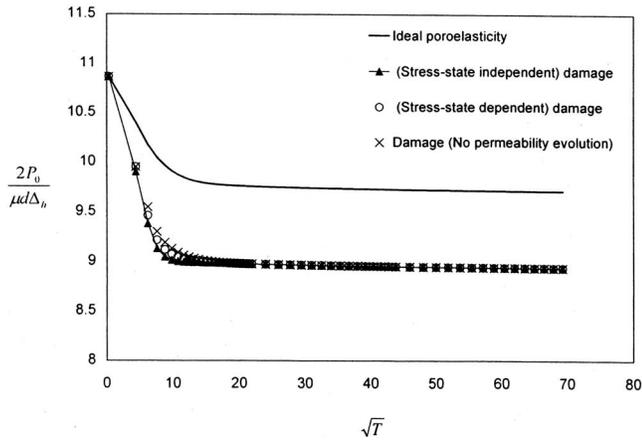
**Fig. 13.** Numerical results for transient translational displacement of rigid rock socket ( $L/d=2.0$ ) embedded in brittle poroelastic half space (impervious interface)
