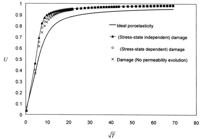
**Fig. 16.** Numerical results for degree of consolidation for rigid rock socket ( $L/d=2.0$ ) embedded in brittle poroelastic half space (impervious interface)
