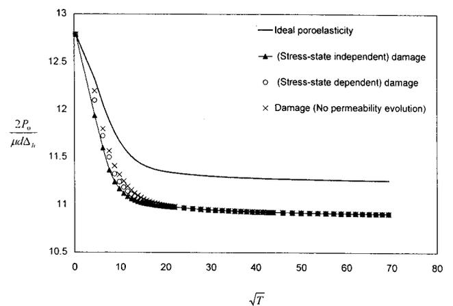
**Fig. 18.** Numerical results for transient translational displacement of rigid rock socket ( $L/d=4.0$ ) embedded in brittle poroelastic half space (impervious interface)
