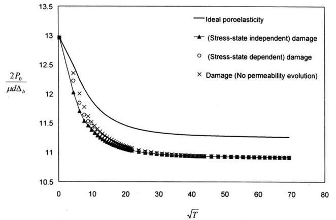
**Fig. 17.** Numerical results for transient translational displacement of rigid rock socket ( $L/d=4.0$ ) embedded in brittle poroelastic half space (pervious interface)
