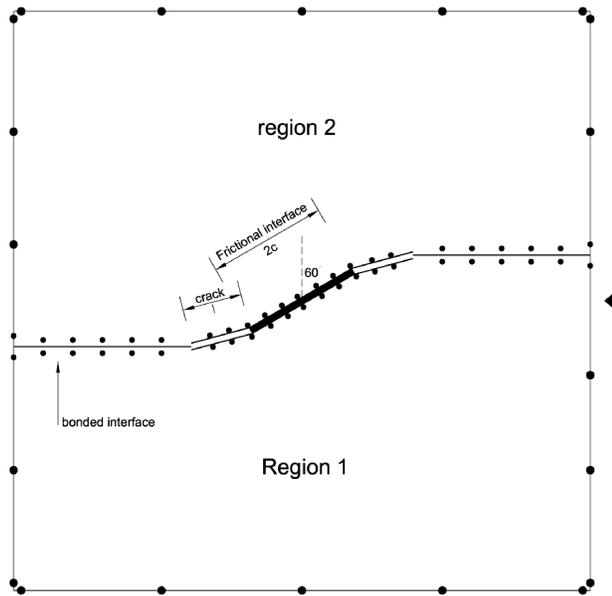
FIG. 3. Boundary element discretizations of the domain.
