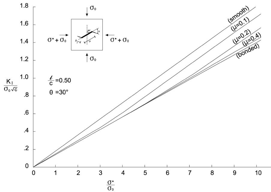
FIG. 8. Mode I stress intensity factor at the crack tip [ $\beta = 60^\circ$ ].
