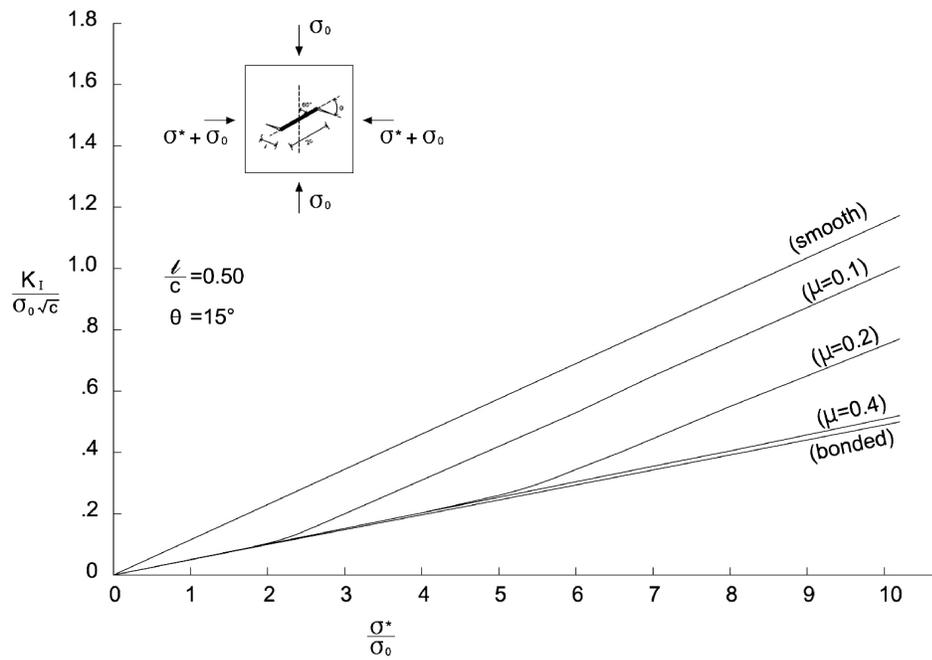
FIG. 5. Mode I stress intensity factor at the crack tip [ $\beta = 60^\circ$ ].
