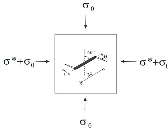
FIG. 1. Wing-cracks extending from interface with Coulomb frictional.
