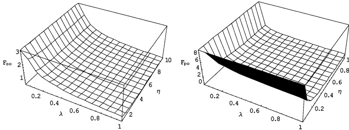
**Figure 3.** Variation of  $F_{oo}/2\pi D$  and  $F_{po}/2\pi D$  with  $\lambda \in (0, 1)$  and  $\eta \in (1, 10)$ .
