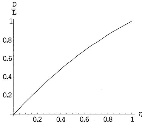
**Figure 4.** Variation of  $D/L$  with  $\eta$  as computed on the basis of equal surface areas between the spheroidal cavity and the cylindrical cavity.
