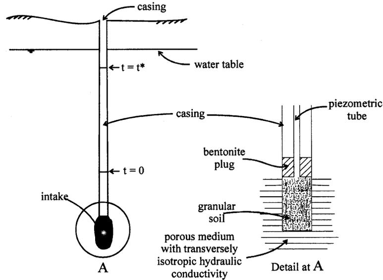
**Figure 1.** Casing test configuration for the in situ determination of the hydraulic properties of geomaterials with low hydraulic conductivity.
