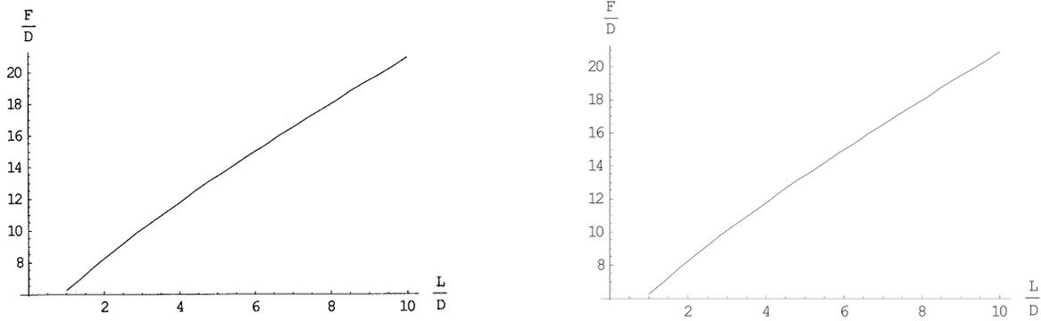
**Figure 5.** Comparisons between Hvorslev's result for the intake shape factor and that derived from the prolate spheroid analysis, where the dimensions are assigned through equivalence of surface areas
