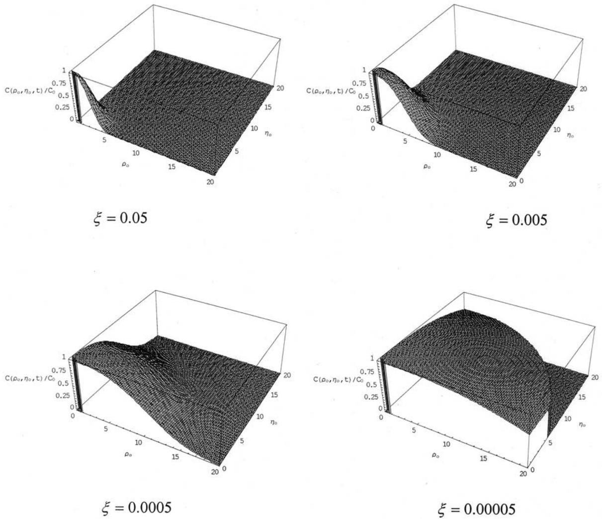
**Figure 13.** The influence of the attenuation coefficient on the pattern of contamination migration from an oblate spheroidal cavity with  $a_0/b_0 = 1/2$  and at time  $t = 10,000$  hours.
