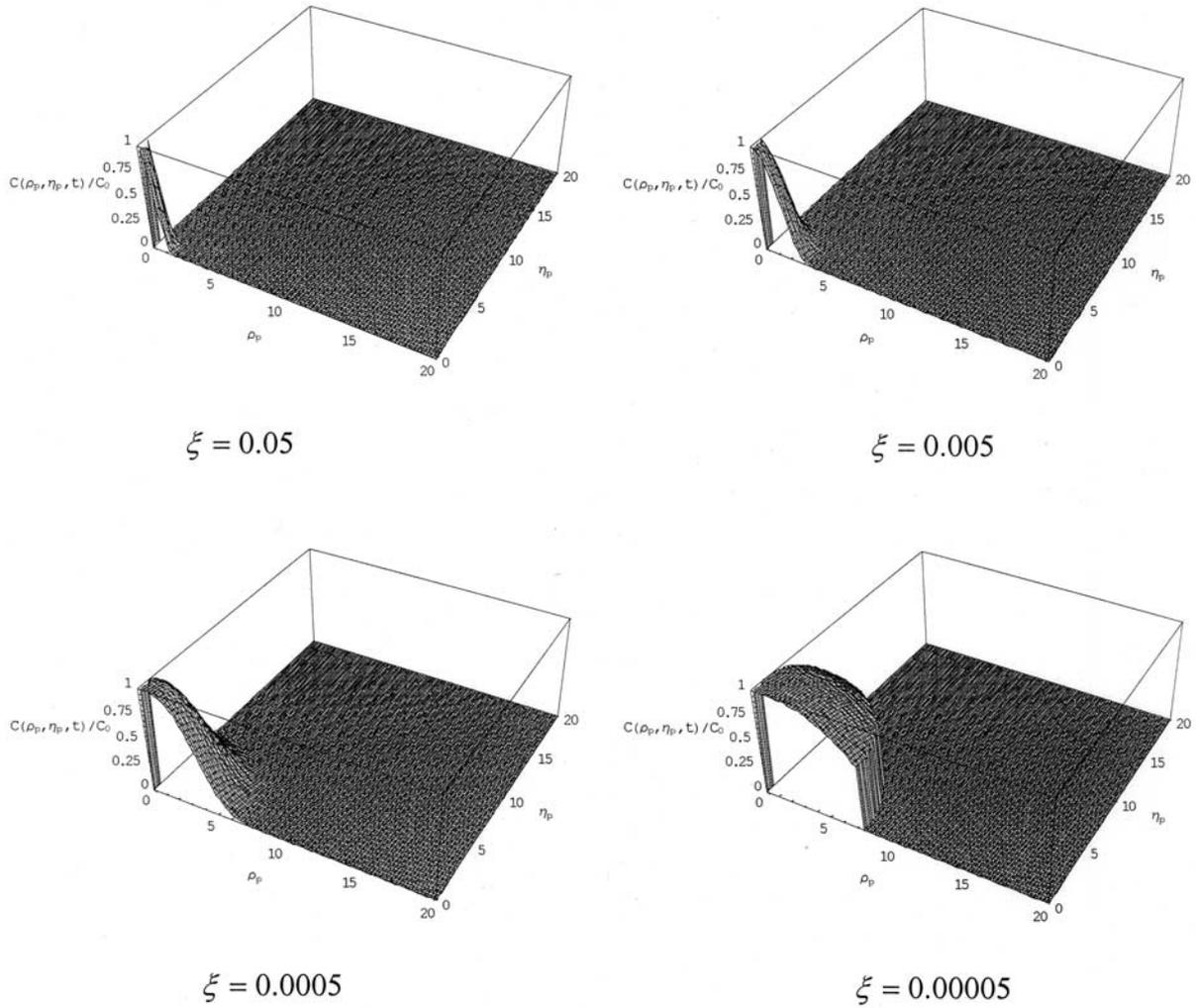
**Figure 10.** The influence of the attenuation coefficient on the pattern of contamination migration from a prolate spheroidal cavity with  $b_p/a_p = 1/8$  and at time  $t = 10,000$  hours.
