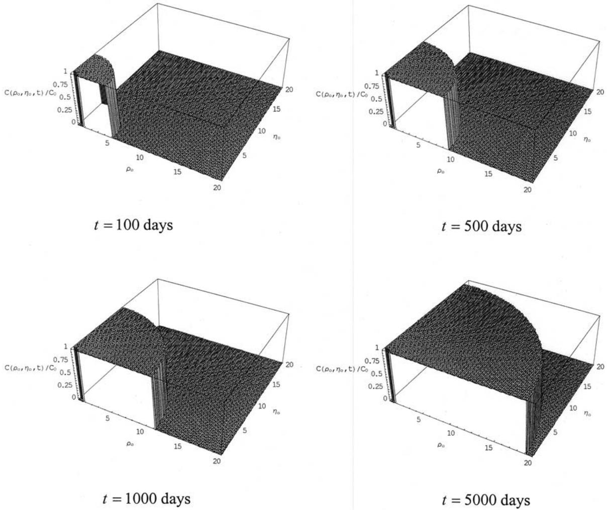
**Figure 5.** Advective transport of the contaminant from an oblate spheroidal cavity with  $a_o/b_o = 1/2$  located in a porous medium with attenuation coefficient  $\xi = 0$ .
