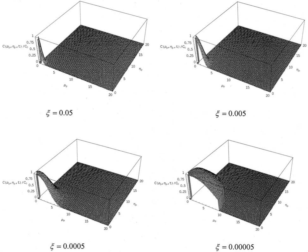
**Figure 11.** The influence of the attenuation coefficient on the pattern of contamination migration from a prolate spheroidal cavity with  $b_p/a_p = 1/2$  and at time  $t = 10,000$  hours.
