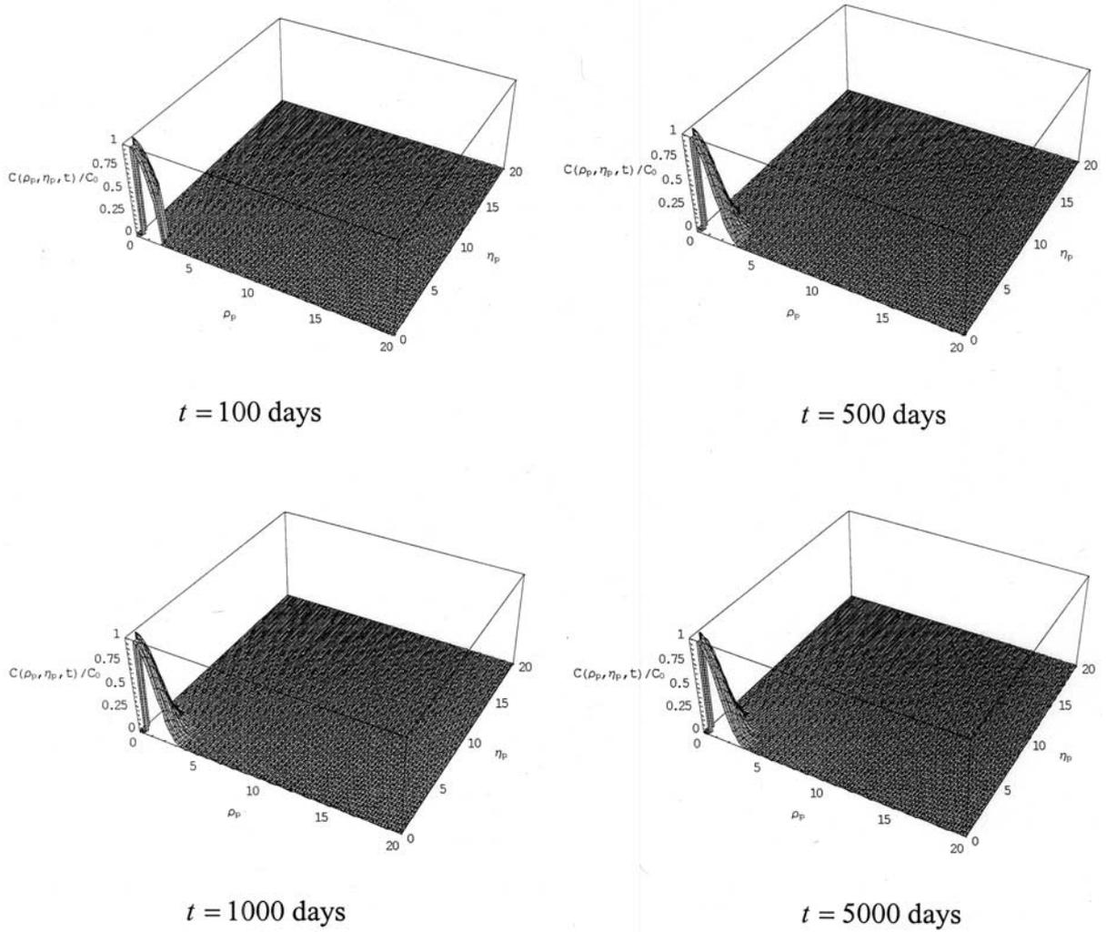
**Figure 7.** Advective transport of the contaminant from a prolate spheroidal cavity with  $b_p/a_p = 1/2$  and located in a porous medium with attenuation coefficient  $\xi = 0.005/\text{day}$ .
