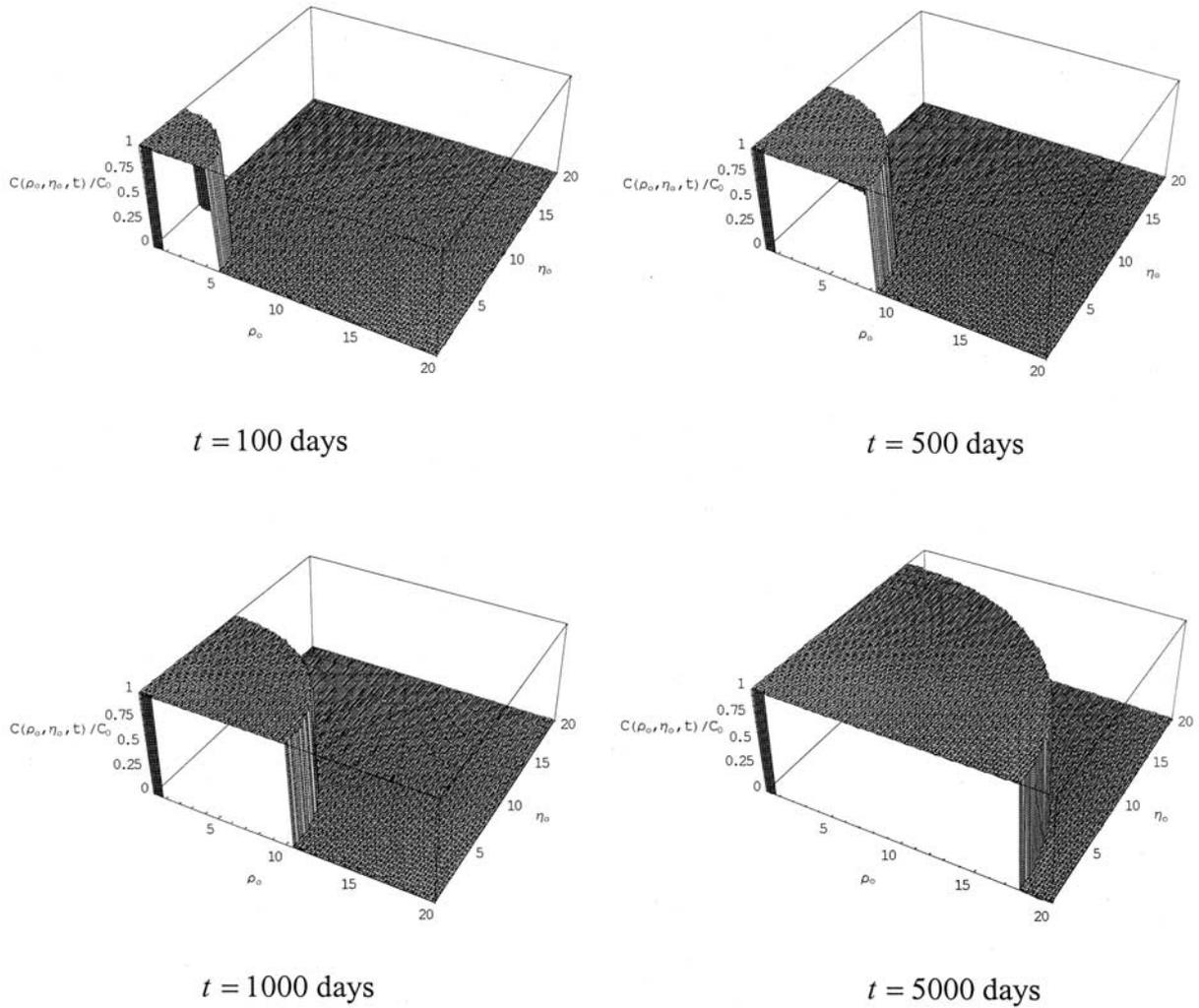
**Figure 4.** Advective transport of the contaminant from an oblate spheroidal cavity with  $a_o/b_o = 1/8$  located in a porous medium with attenuation coefficient  $\xi = 0$ .
