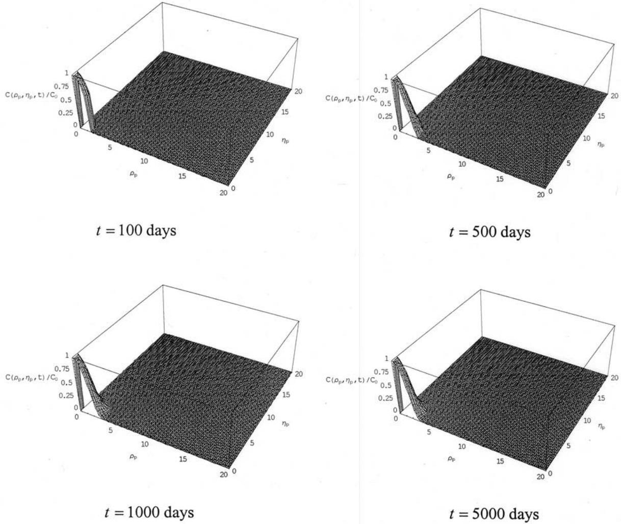
**Figure 6.** Advective transport of the contaminant from a prolate spheroidal cavity with  $b_p/a_p = 1/8$  and located in a porous medium with attenuation coefficient  $\xi = 0.005/\text{day}$ .
