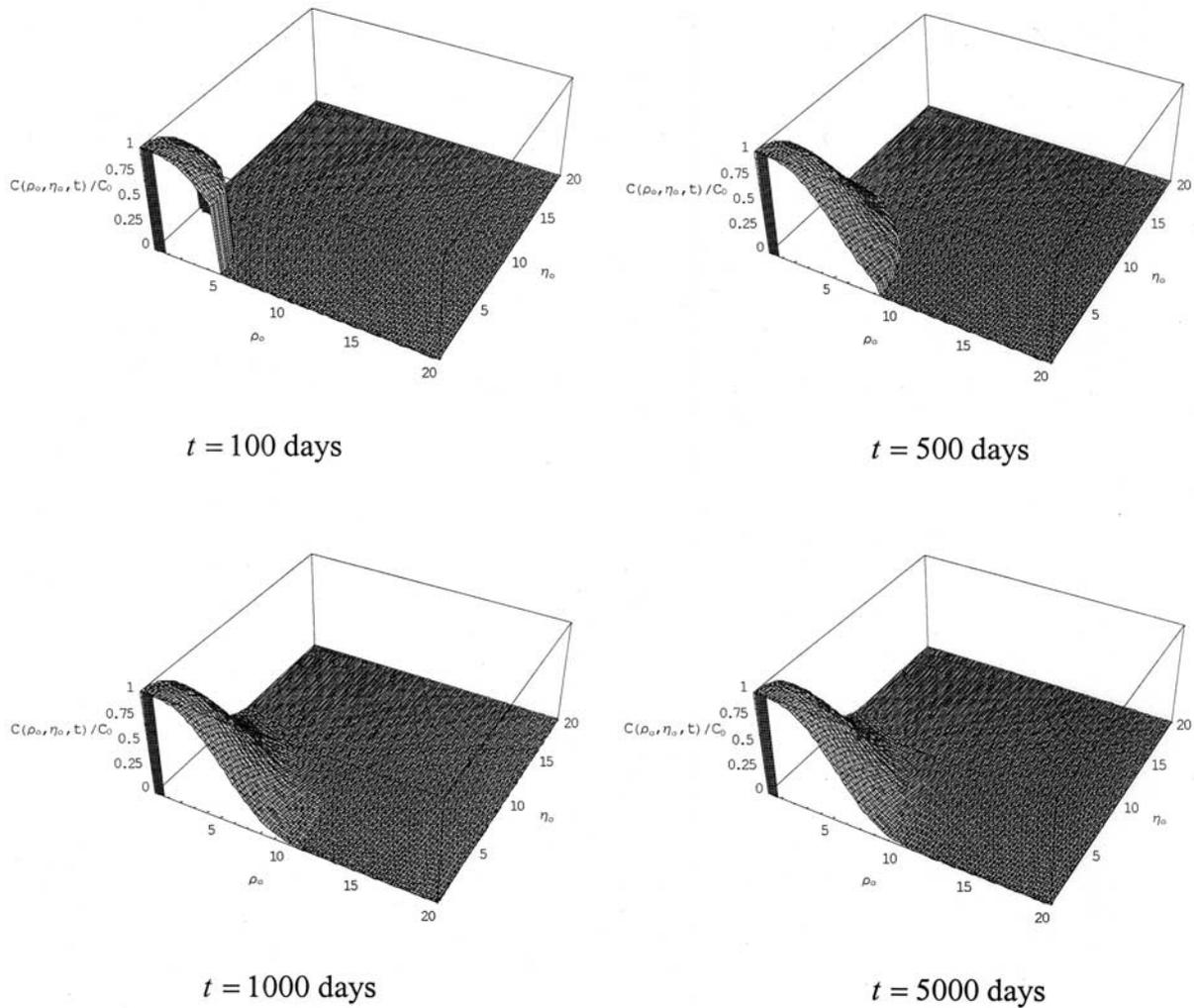
**Figure 8.** Advective transport of the contaminant from an oblate spheroidal cavity with  $a_o/b_o = 1/8$  and located in a porous medium with attenuation coefficient  $\xi = 0.005/\text{day}$ .
