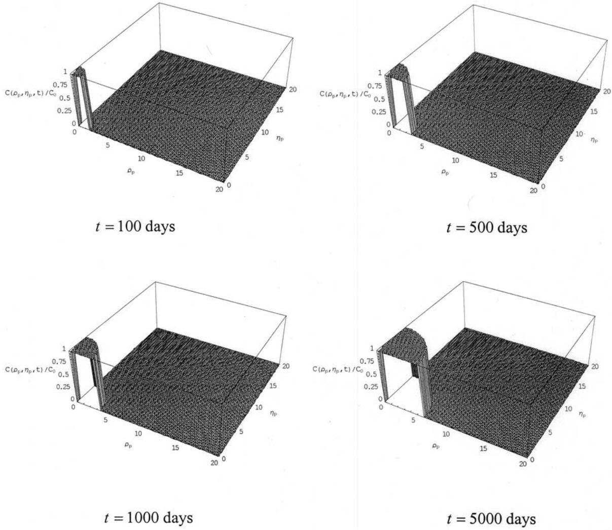
**Figure 2.** Advective transport of the contaminant from a prolate spheroidal cavity with  $b_p/a_p = 1/8$  located in a porous medium with attenuation coefficient  $\xi = 0$ .
