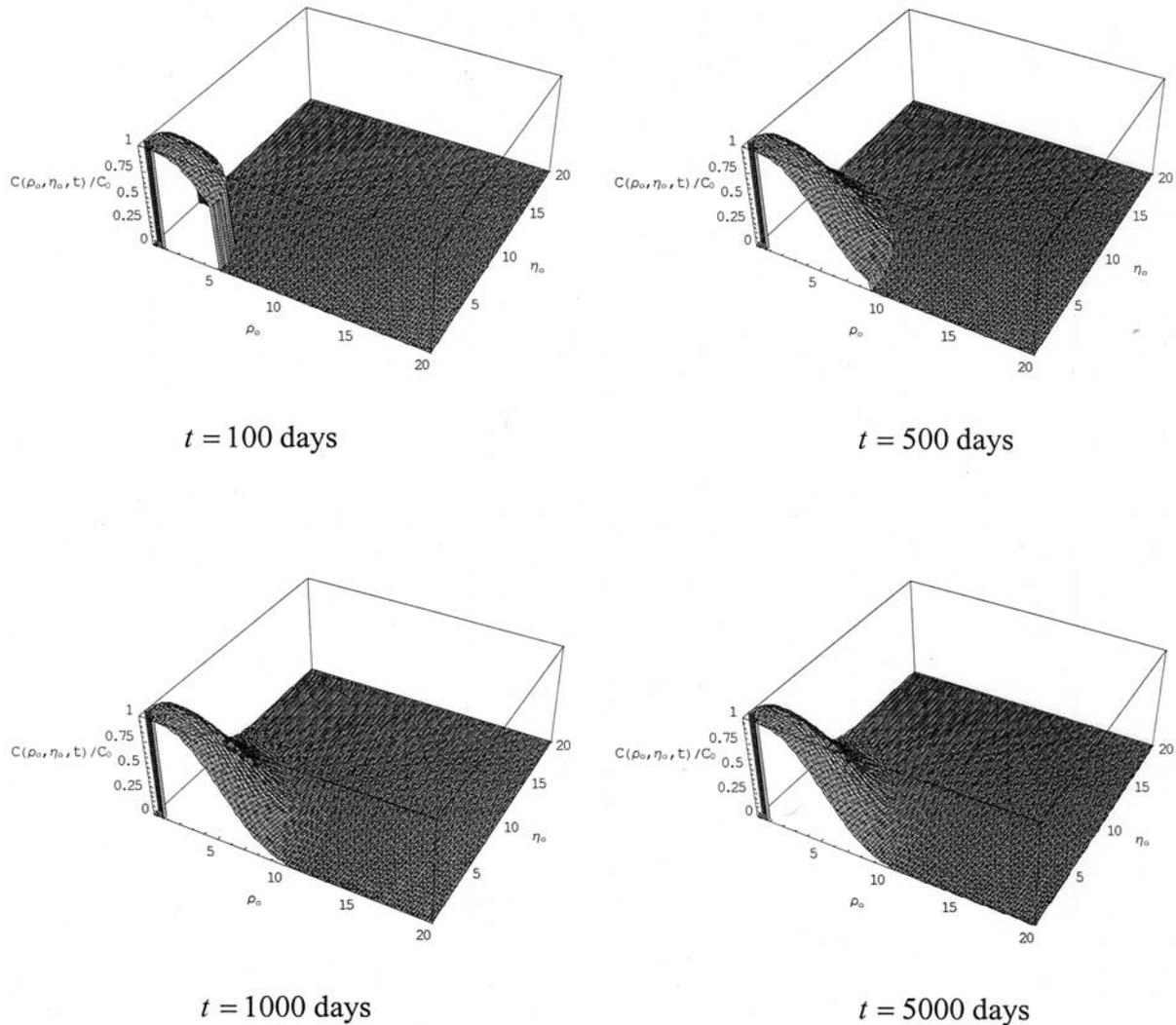
**Figure 9.** Advective transport of the contaminant from an oblate spheroidal cavity with  $a_o/b_o = 1/2$  and located in a porous medium with attenuation coefficient  $\xi = 0.005/\text{day}$ .
