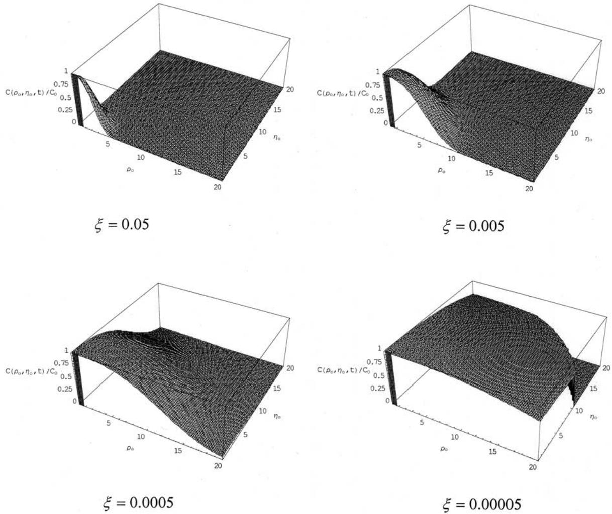
**Figure 12.** The influence of the attenuation coefficient on the pattern of contamination migration from an oblate spheroidal cavity with  $a_o/b_o = 1/8$  and at time  $t = 10,000$  hours.
