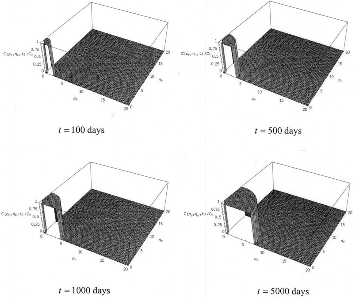
**Figure 3.** Advective transport of the contaminant from a prolate spheroidal cavity with  $b_p/a_p = 1/2$  located in a porous medium with attenuation coefficient  $\xi = 0$ .
