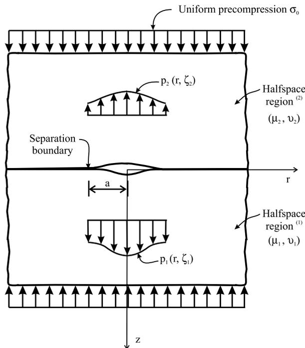
Fig. 1. Unilateral contact at a pre-compressed bimaterial elastic interface.
