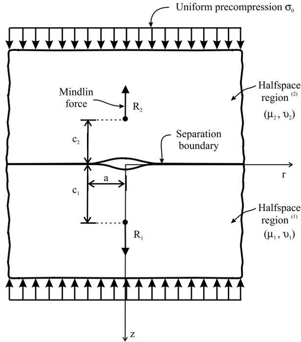
Fig. 4. Separation at the pre-compressed bimaterial elastic interface by unequal Mindlin forces applied at the interior of the halfspace regions.
