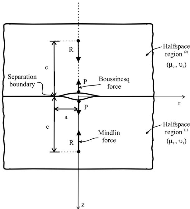
Fig. 5. Bimaterial elastic interface pre-compressed by equal Mindlin forces and separation induced by identical Boussinesq forces applied at the interface.
