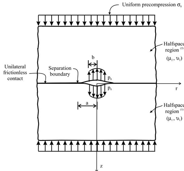
Fig. 2. Separation at the pre-compressed bimaterial elastic interface by tractions applied at the interface.
