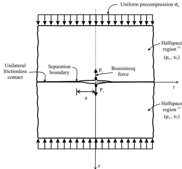
Fig. 3. Separation at the pre-compressed bimaterial elastic interface by unequal Boussinesq forces applied at the interface.
