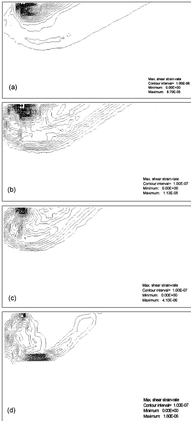
**FIG. 3.** Contours of Maximum Shear Strain Rate for  $N_c$ : (a)  $\psi = \phi$ ; (b)  $\psi = 2\phi/3$ ; (c)  $\psi = \phi/3$ ; (d)  $\psi = 0$
