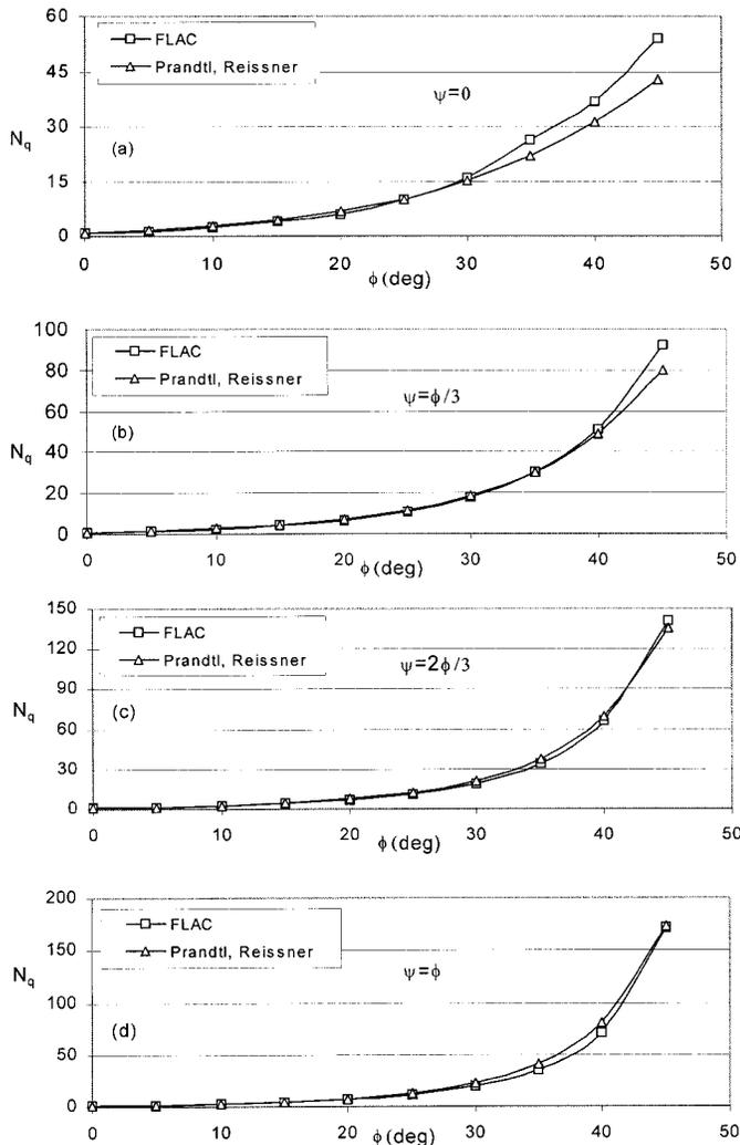
**FIG. 5.** Comparison of  $N_q$ : (a)  $\psi = 0$ ; (b)  $\psi = \phi/3$ ; (c)  $\psi = 2\phi/3$ ; (d)  $\psi = \phi$
