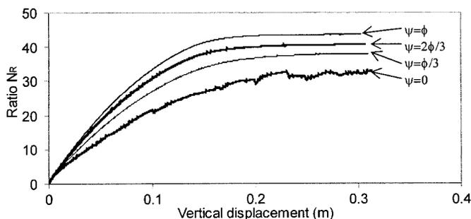
**FIG. 1.** Ratio  $N_R$  versus Vertical Displacement for Different Dilation Angle  $\psi = \phi, 2\phi/3, \phi/3, \text{ and } 0$
