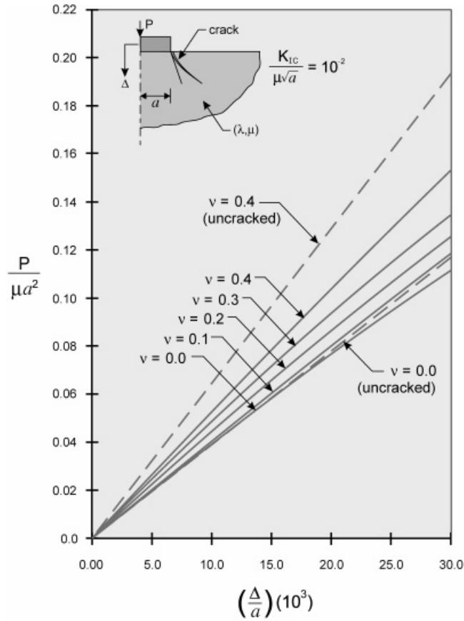
Figure 8. Influence of conoidal cracks development on the displacement behaviour of the rigid smooth indenter. [Starter crack orientation determined from consideration of stress state (see Figure 4)]
