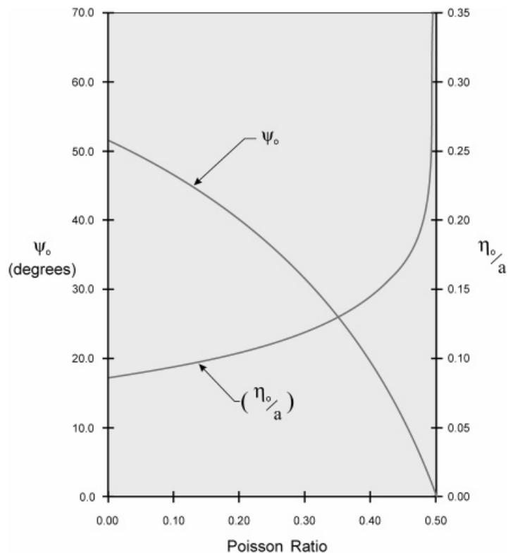
Figure 4. Location of the point of maximum tensile stress at the boundary of the rigid, smooth indenter (co-ordinates  $(\eta_0/a)$  and  $\psi$  are defined in Figure 3)
