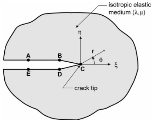
Figure 2. Crack tip geometry and node locations
