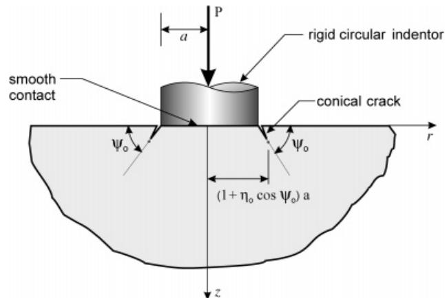
Figure 5. Starter crack configuration for the computational modelling of crack extension
