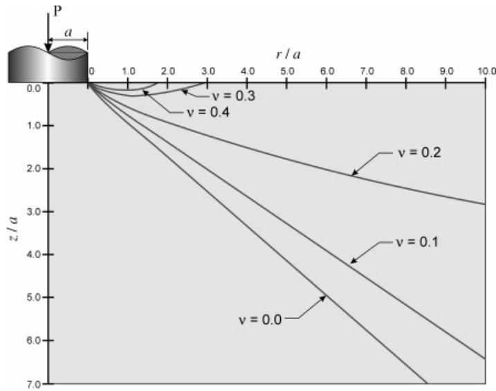
Figure 6. Pattern of conoidal crack development at the boundary of the rigid smooth indenter. (Starter crack orientation determined from Figure 4)
