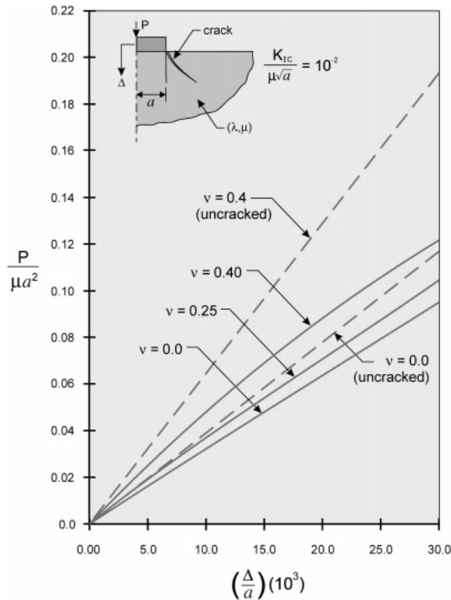
Figure 9. Influence of conoidal crack development on the rigid smooth indenter. (Starter crack normal to the plane boundary)
