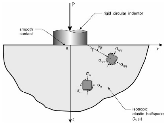
Figure 3. Local stress field at the boundary of the rigid circular indenter
