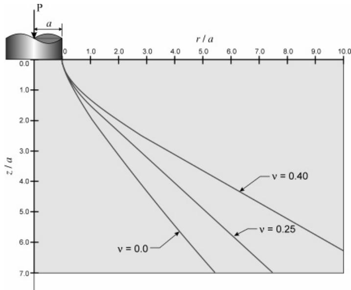
Figure 7. Pattern of conoidal crack development at the boundary of the rigid smooth indenter. (Starter crack normal to the plane boundary)
