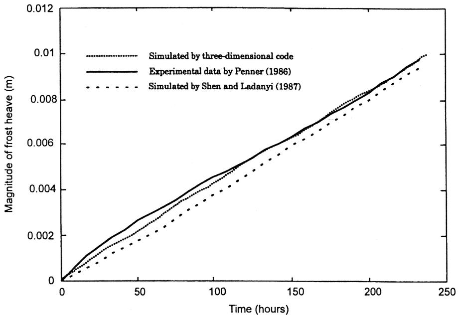
Fig. 2. Frost heave generation in a sample of silty clay.
