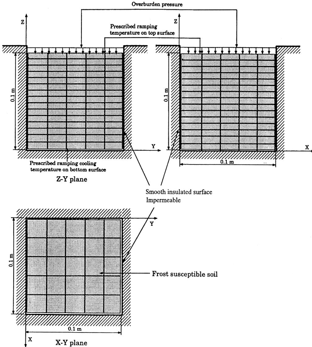
Fig. 1. Finite element discretization of the cuboidal element.
