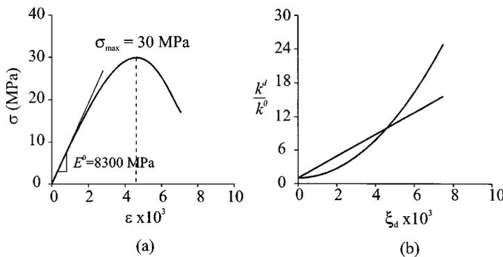
Figure 4. The stress–strain behaviour and permeability evolution of saturated geomaterial
