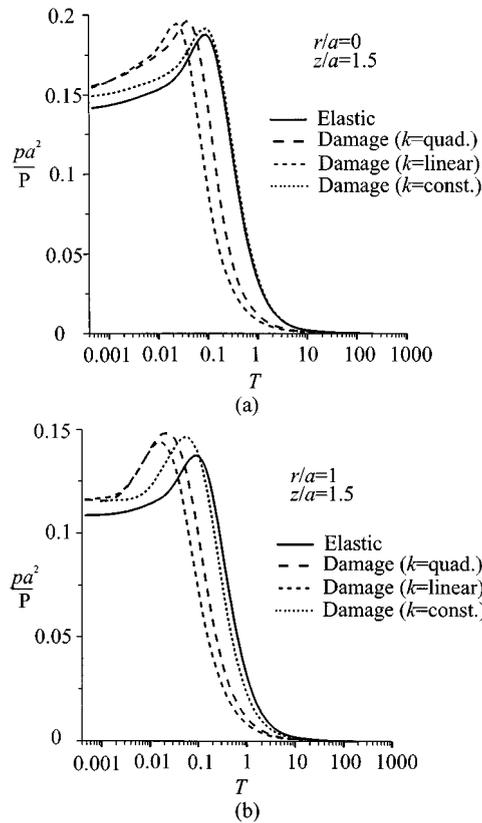
Figure 7. Pore pressure evolution at different depths
