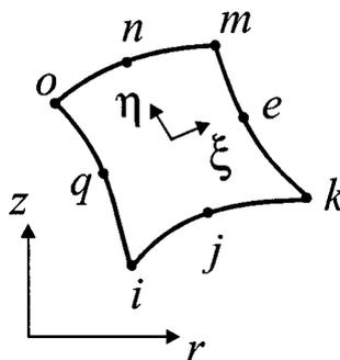
Figure 2. Solid isoparametric element
