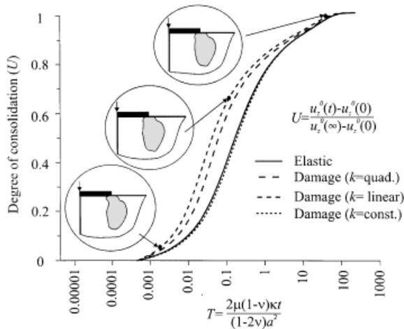
Figure 6. Degree of consolidation and evolution of damaged zone (where  $D/D_c > 0.05$ ) with time
