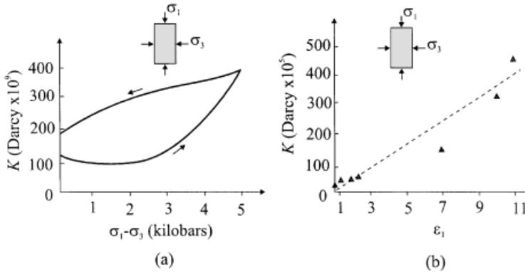
Figure 3. Permeability evolution in saturated geomaterials (a) after Zoback and Byerlee;<sup>11</sup> and (b) after Shiping *et al.*<sup>12</sup>
