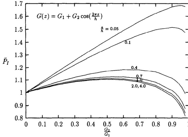
Fig. 4. Inclusion problem : variation of the nondimensional force  $\bar{P}_1$  with respect to the ratio  $G_2/G_1$  for  $\nu = 0.3$  and various values of  $a/h$ .
