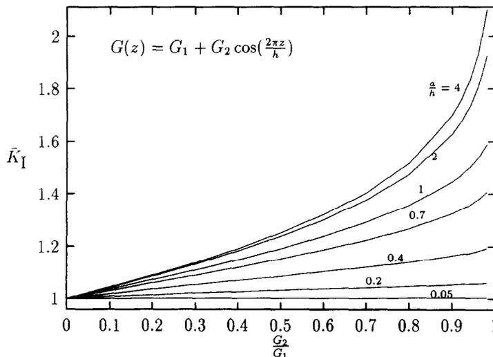
Fig. 6. Crack problem: variation of the nondimensional stress intensity factor  $\bar{K}_I$  with respect to  $G_2/G_1$  for  $\nu = 0.3$  and various values of  $a/h$ .
