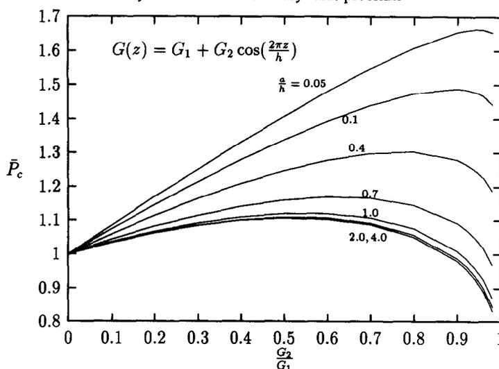
Fig. 2. Contact problem: variation of the nondimensional force  $\bar{P}_c$  with respect to the ratio  $G_2/G_1$  for  $\nu = 0.3$  and various values of  $a/h$ .
