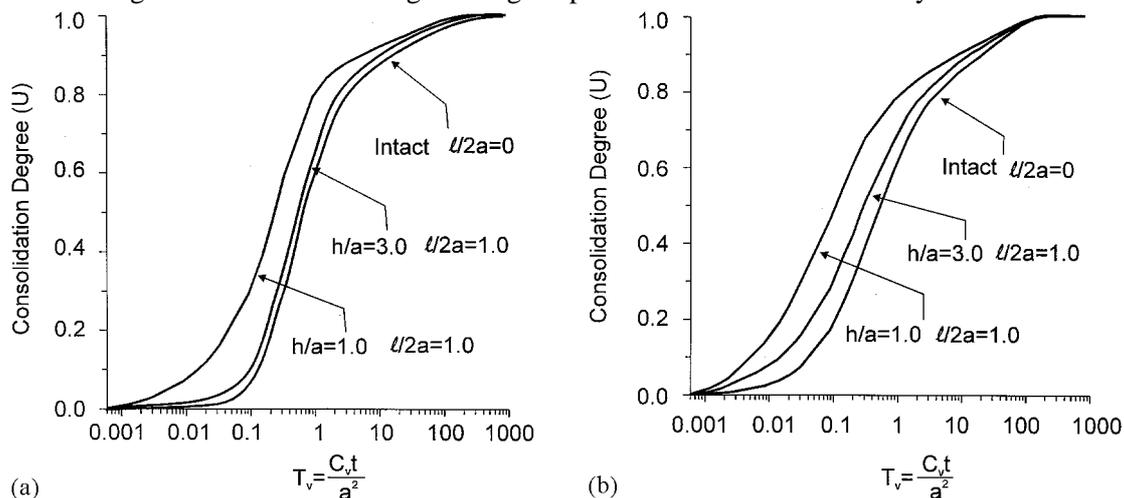
Figure 11. Consolidation response of a poroelastic half-space containing a flat penny-shaped co-axial crack; (a) impermeable bonded interface; and (b) permeable bonded interface.
