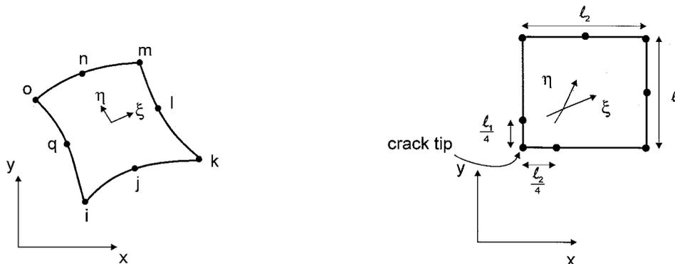
Figure 3 (a) Plane isoparametric element; and (b) Quarter point isoparametric element.
