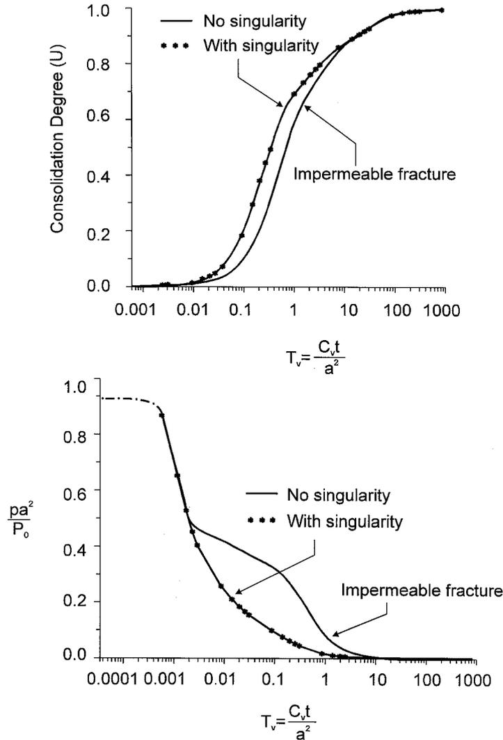
Figure 8. Effect of crack tip singularity and permeability of crack face for a cylindrical crack of  $\ell/a = 1$  and  $b/a = 1$  on; (a) Consolidation settlement of indenter; and (b) Pore pressure at crack tip.
