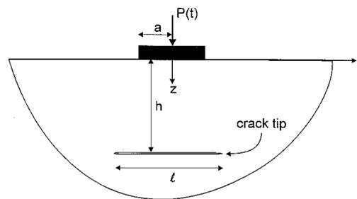
*Figure 2.* Indentation of a poroelastic half-space containing a flat penny-shaped co-axial crack.
