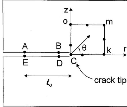
Figure 4. Details of the crack tip and node arrangement for computation of the stress intensity factors.
