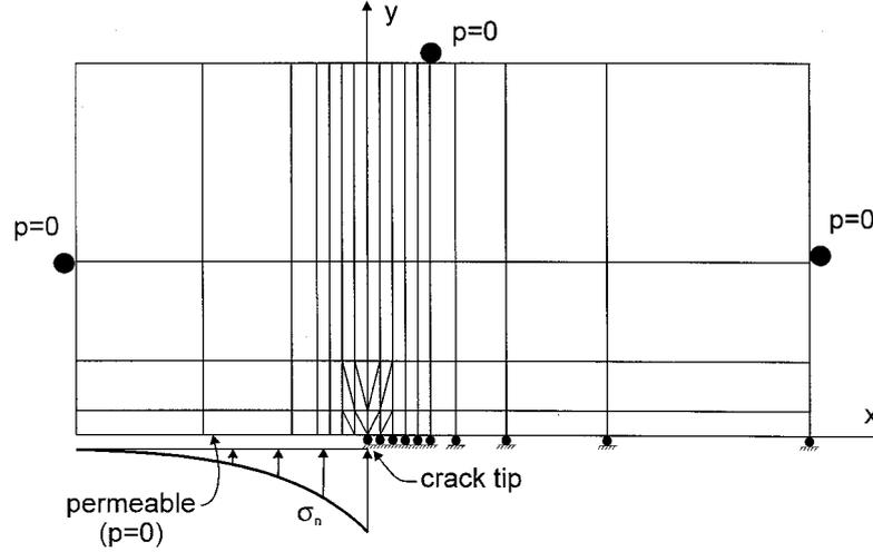
Figure 5. Finite element discretization of a semi infinite crack in a poroelastic medium.
