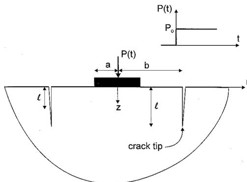
*Figure 1.* Indentation of a poroelastic half-space containing a cylindrical crack.
