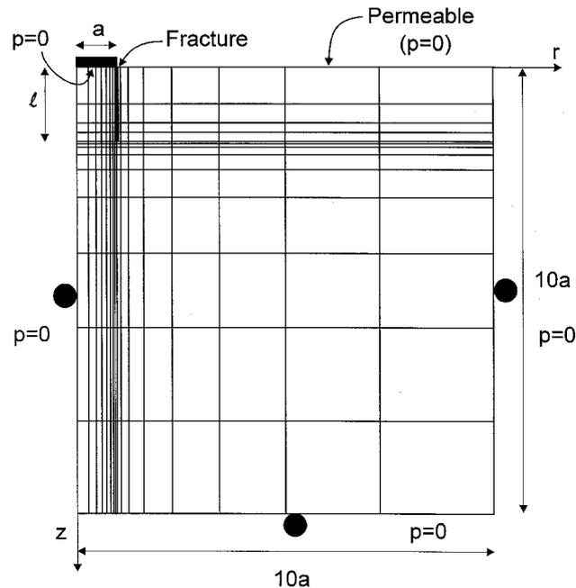
Figure 7. Finite element discretization of the poroelastic medium containing a cylindrical crack of  $\ell/a = 2$  and  $b/a = 1$ .
