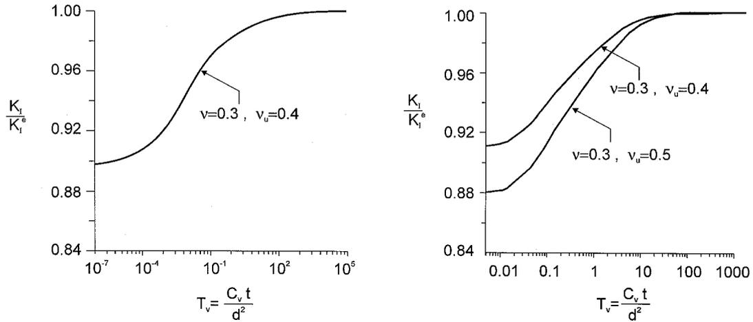
Figure 6. Time dependent variation of the stress intensity factor  $K_I$  for semi infinite crack with permeable faces; (a) Atkinson and Craster (1991) and Craster and Atkinson (1996); and (b) Finite element analysis.
