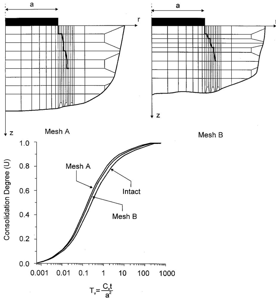
Figure 10. (a) Finite element discretization of quasi-static crack extension problem in a poroelastic medium with  $\nu_u = 0.3$  and  $\nu = 0.1$ ; and (b) Consolidation settlement of indenter.
