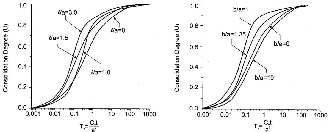
Figure 9. Consolidation response of a poroelastic half-space containing a cylindrical crack; (a) Effect of crack length for  $b/a = 1$ ; and (b) Effect of location of crack for  $\ell/a = 3$ .
