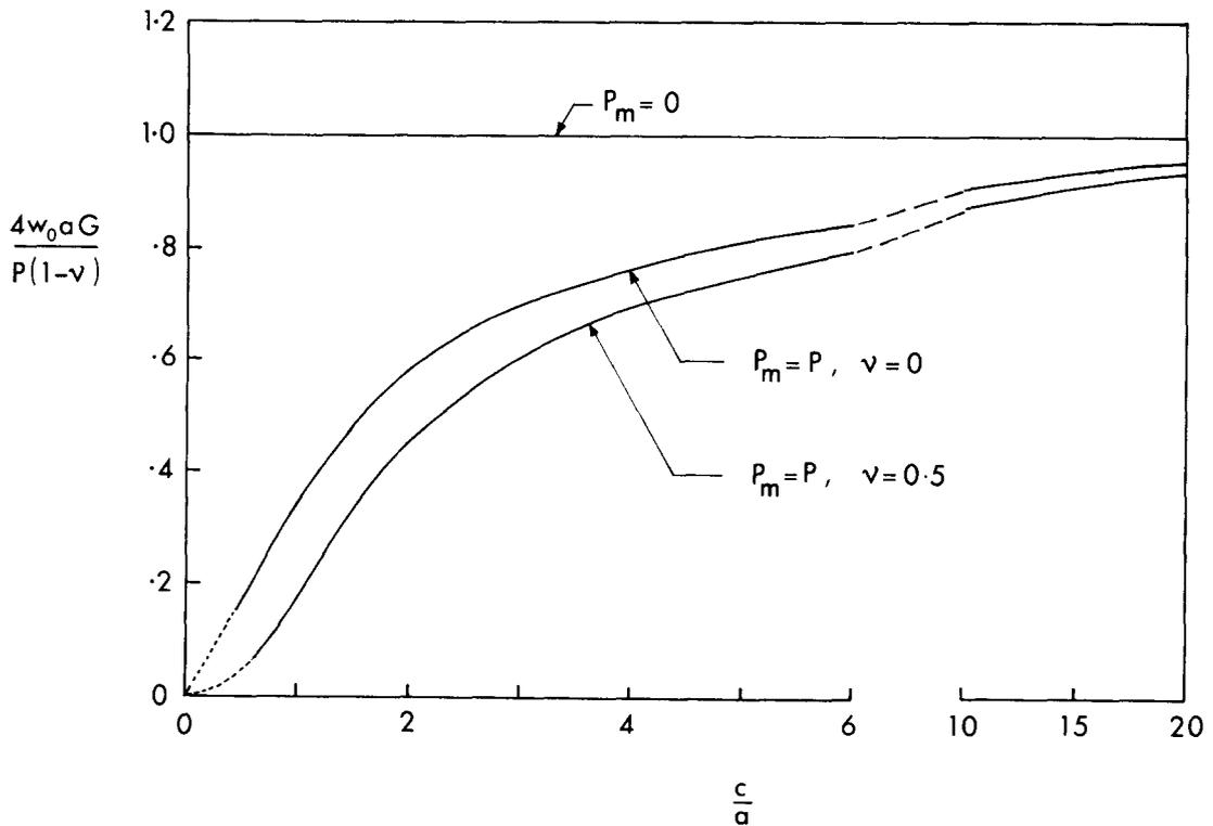
Fig. 3. The influence of the location of the Mindlin force on the deflection of the rigid circular punch.
