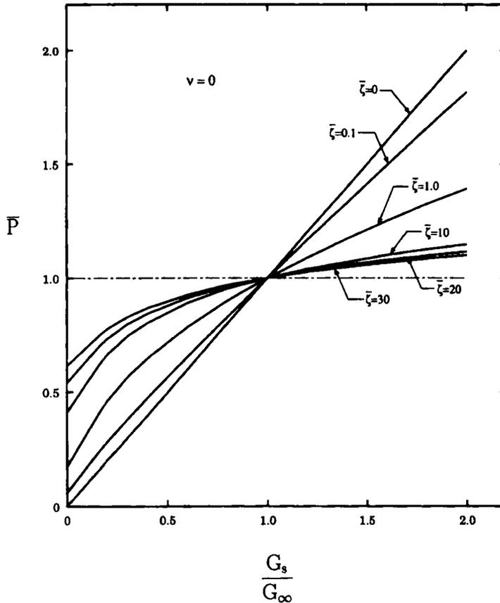
Figure 2. Axial stiffness of a rigid circular foundation on a non-homogeneous elastic half-space
