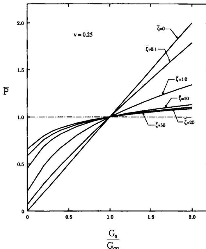
Figure 3. Axial stiffness of a rigid circular foundation on a non-homogeneous elastic half-space
