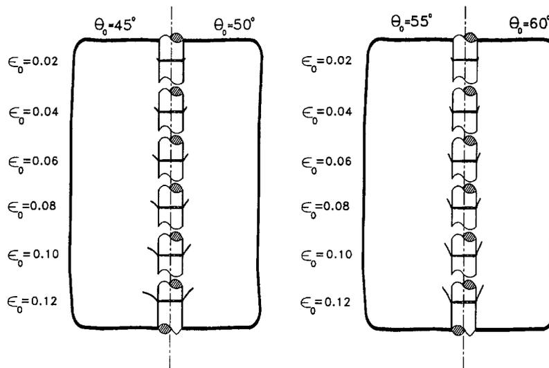
Fig. 6 Matrix crack extension at a cracked fiber location: elemental conical crack oriented at an arbitrary inclination to the fiber
