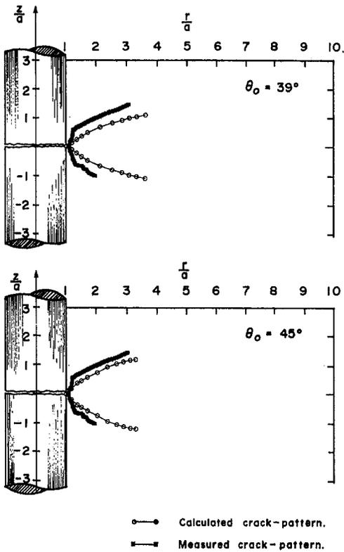
Fig. 10 Matrix crack extension due to the growth of conoidal cracks: a comparison of experimental results and computational estimates (accurate experimental data)
