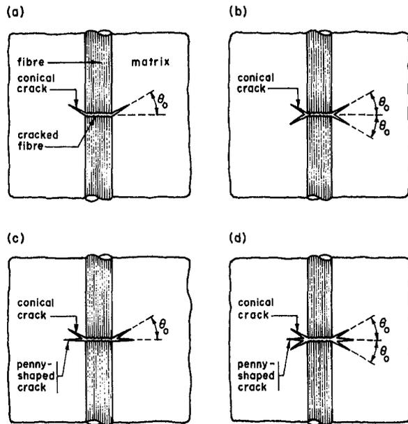
Fig. 4 Elemental matrix crack configurations at cracked fiber locations; (a) elemental conical crack, (b) elemental conical cracks which are symmetrically located about the plane of the cracked fiber, (c) a combination of an elemental penny-shaped crack and a single elemental conical crack, (d) a combination of an elemental penny-shaped crack and symmetrically placed elemental conical cracks, ( $\theta_0 = \pi/2 - \varphi_0$ )
