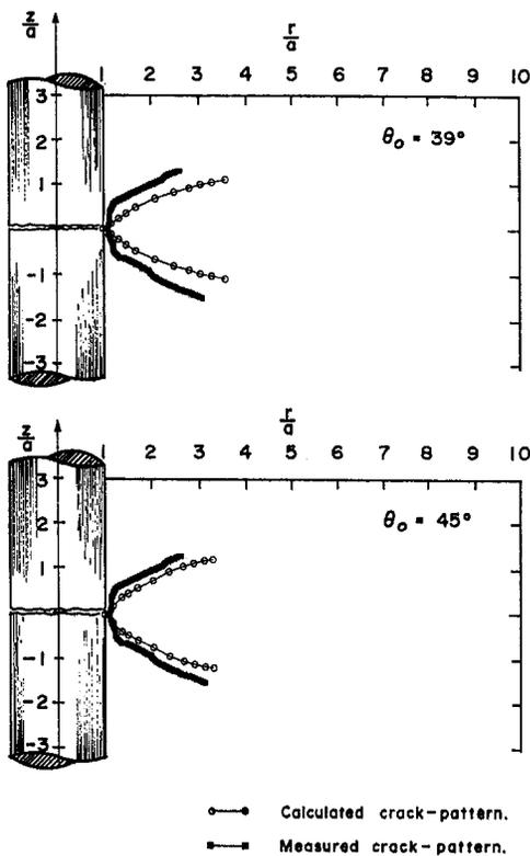
Fig. 11 Matrix crack extension due to the growth of conoidal cracks: a comparison of experimental results and computational estimates (approximate experimental data)
