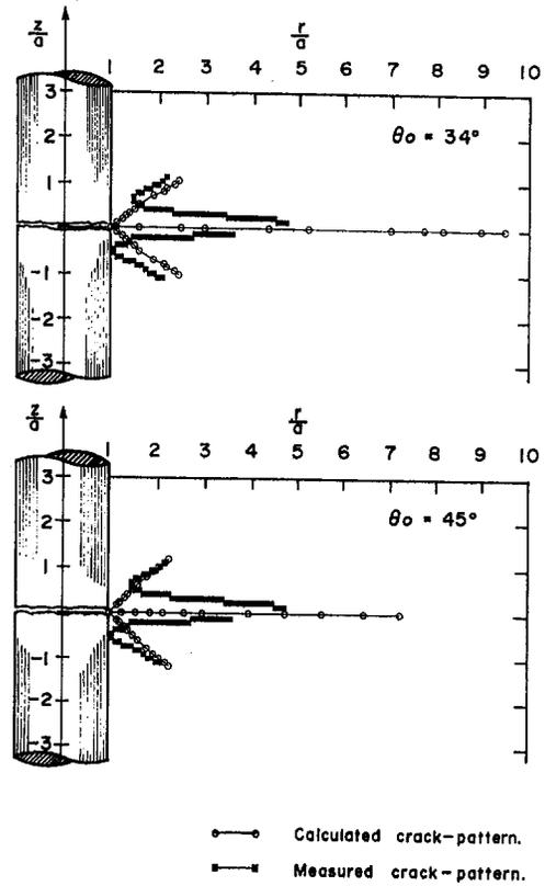
Fig. 12 Matrix crack extension due to the simultaneous growth of conoidal and penny-shaped cracks: a comparison of experimental results and computational estimates (accurate experimental data)
