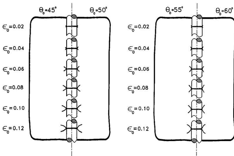
Fig. 7 Matrix crack extension at a cracked fiber location: elemental conical cracks symmetrically placed about the plane of crack fiber
