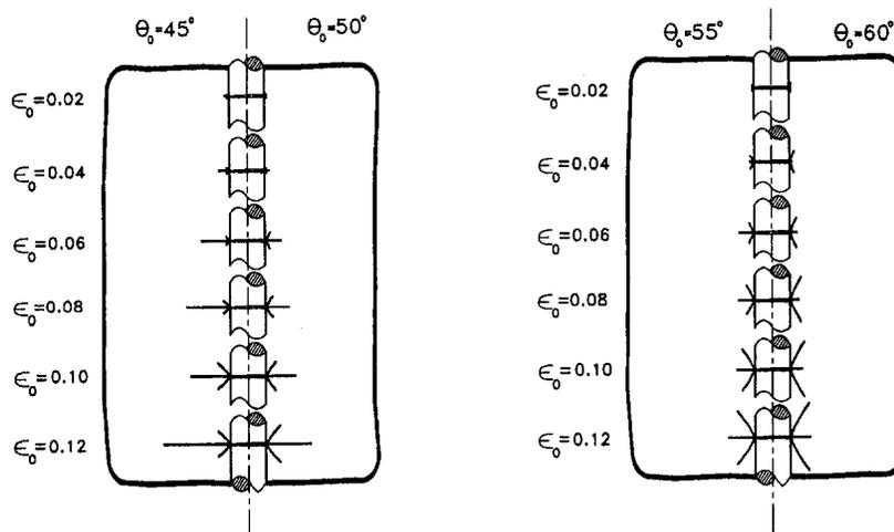
Fig. 9 Matrix crack extension at a cracked fiber location: a combination of an elemental penny-shaped crack and symmetrically placed elemental conical cracks
