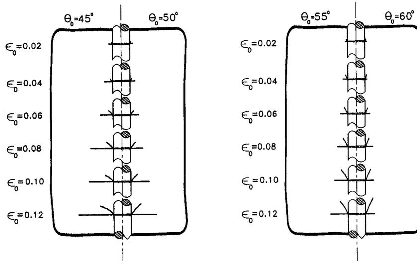
Fig. 8 Matrix crack extension at a cracked fiber location: a combination of an elemental penny-shaped crack and an elemental conical crack
