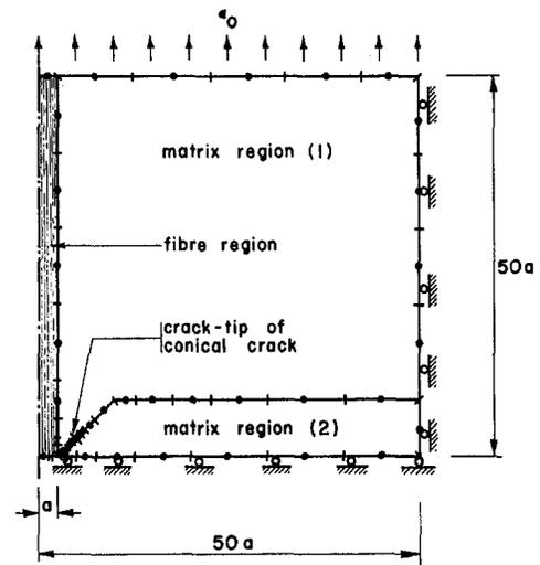
Fig. 5 Boundary element discretization used in the numerical modeling of the fragmentation test
