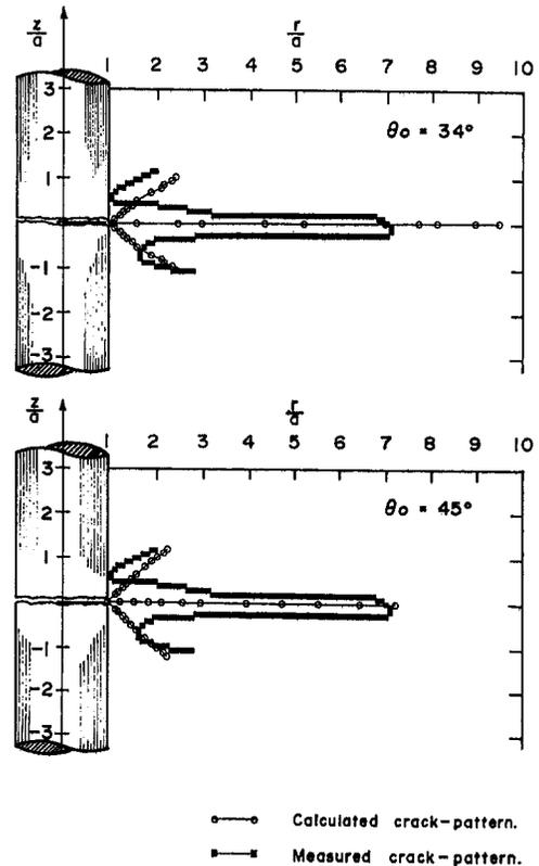
Fig. 13 Matrix crack extension due to the simultaneous growth of conoidal and penny-shaped cracks: a comparison of experimental results and computational estimates (approximate experimental data)
