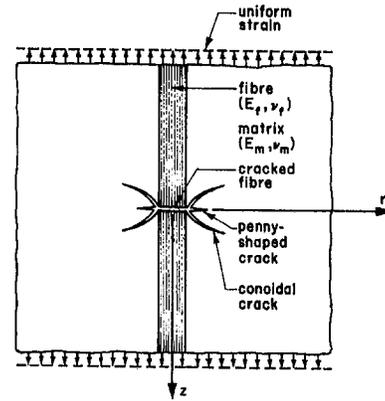
Fig. 1 The axisymmetric model of the fragmentation tests for an embedded fiber
