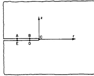
Fig. 2 Detail at the crack tip. Node arrangement for the computation of the stress intensity factor.
