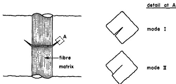
Fig. 3 Fracture modes at tip of matrix crack
