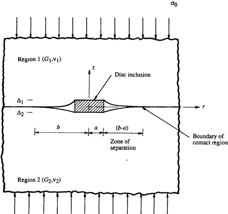
FIG. 1. The disc inclusion embedded between two dissimilar elastic half-spaces
