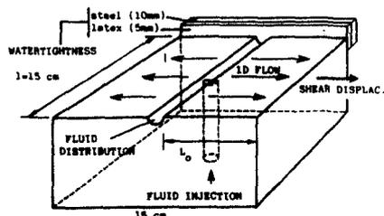
1b. The rock joint sample prepared for a 1D flow.
