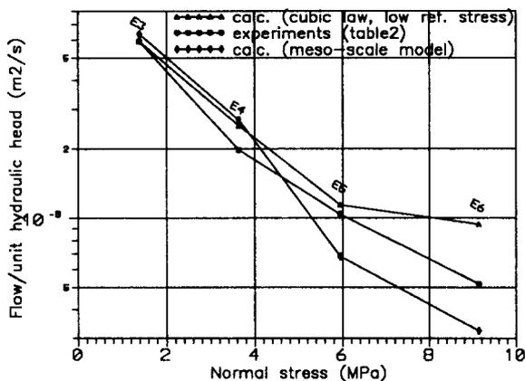
Fig.5. Sample L2 under normal stress, conductivity experiments and simulations. Meso-scale model:  $n = 0.21$ ,  $e_{hmo} = 0.207$  mm, mean residual =  $4e-9$  m<sup>2</sup>/s.
