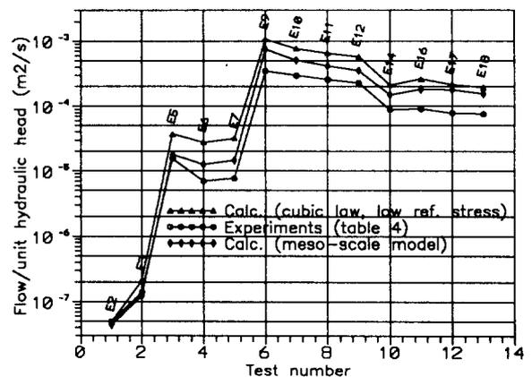
Fig.7. Sample L1 under shear displacements and normal stress, conductivity experiments and simulations. Meso-scale model:  $n = 0.07$ ,  $e_{hmo} = 0.297$  mm, mean residual =  $7e-5$  m<sup>2</sup>/s.
