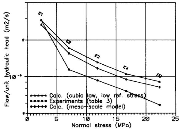
Fig.6. Sample G16 under normal stress, hydraulic conductivity experiments and simulations. Meso-scale model:  $n = 0.09$ ,  $e_{hmo} = 0.165$  mm, mean residual =  $2e-7$  m<sup>2</sup>/s.
