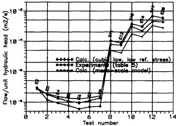
Fig. 8. Sample G16 under shear displacements and normal stress, hydraulic conductivity experiments and simulations. Meso-scale model:  $n = 0.30$ ,  $e_{hmo} = 0.270$  mm, mean residual =  $3e-5$  m<sup>2</sup>/s
