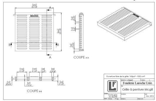
.2 McGill is the owner of the mold, stored at Fonderie Laroche, for a 750x750 cast iron manhole cover, with hinge. A space for a descriptive inscription is available, such as "PLUVIAL", "SANITAIRE" or other as approved by McGill:
