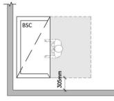
.4 Maintain a distance of 305mm to columns to avoid disturbance to BSC airflow. Columns at a distance of 305mm can aid in defining traffic routes:
