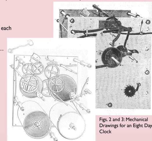
Figs. 2 and 3: Mechanical Drawings for an Eight Day Clock
