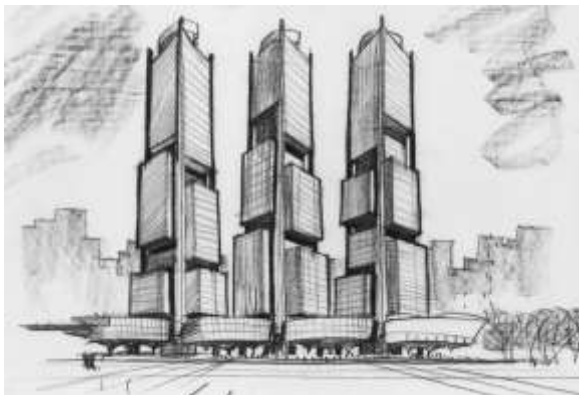
Fig 13 The towers are depicted as an assembly of irregular, powerful blocks held together by the corner columns
