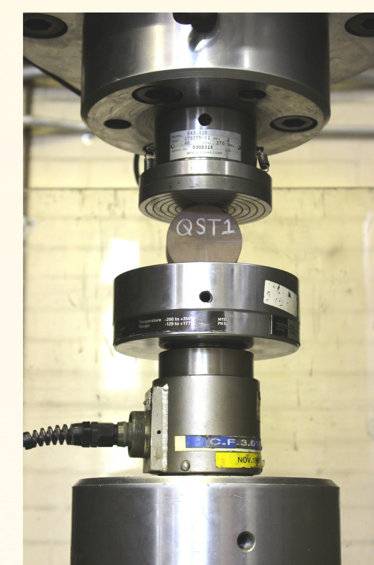
Figure 3: Set up for brazilian test
