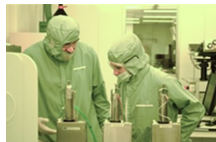
A batch of wafers are entering the oxidation furnace.
