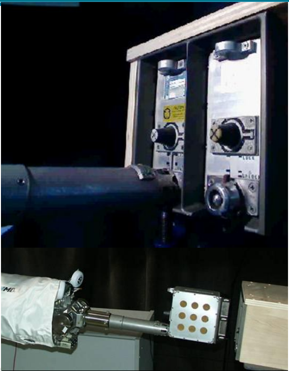
Practicing 'what-ifs' in the lab with the 1g compatible SPDM-GT for the RPCM changeout
