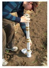
They measure the soil water content by measuring the soil bulk permittivity or dielectric constant
