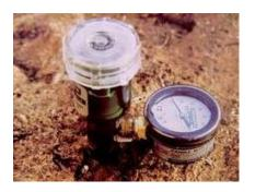
• Consist of a sealed water-filled plastic tube with a ceramic cup at one end and negative pressure gauge at the other.
