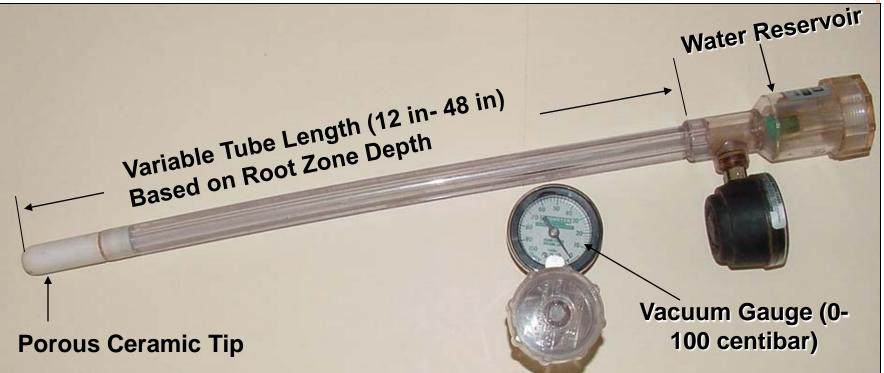
The tensiometer is one of the oldest and most widely used instruments for irrigation scheduling around the world
