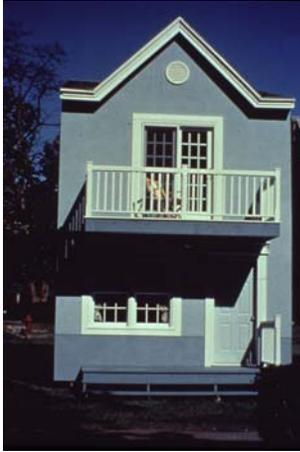
A single family narrow-front townhouse. Spaces can be left unpartitioned for the occupant to “grow” into when means become available. Cost savings resulted from the dwelling’s small size and simplicity, and lowering of cost and infrastructure.
