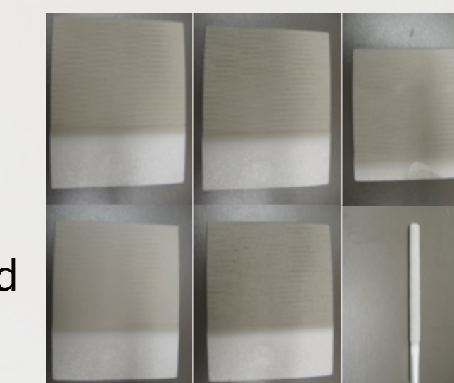
Figure 8. Cold spray deposited coating of composite 316L and pure iron powders onto aluminum substrate
