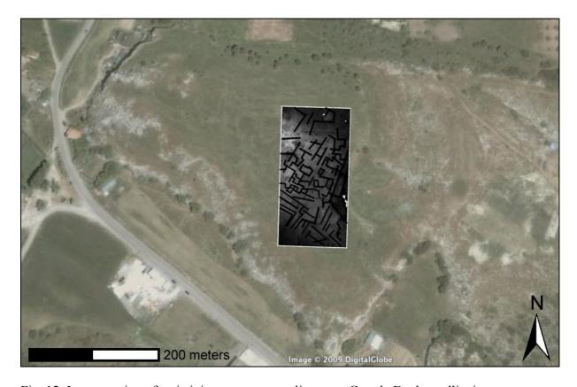
Fig. 12. Interpretation of resistivity survey anomalies, over Google Earth satellite imagery.
