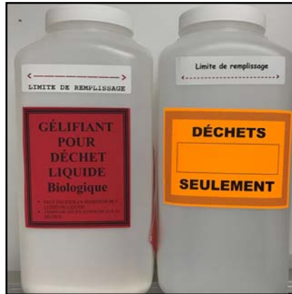
Figure 6: Waste containers for biological and miscellaneous waste red label for biological waste / orange label for miscellaneous waste
