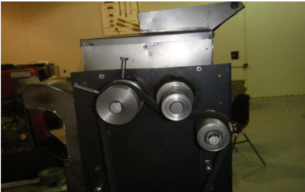
Figure 41 - Rubber Roller and Idler Pulleys
