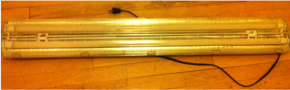
Figure 8. The final prototype consists of an IP65 Linear Fluorescent Fixture (Thomas & Betts, 2013), 2 x 18 Watt LED lamps (Intertek Group, 2013), a dual layer silicone caulking seal, a reduced surface area hard plastic cover, and a retrofitted wiring system.
