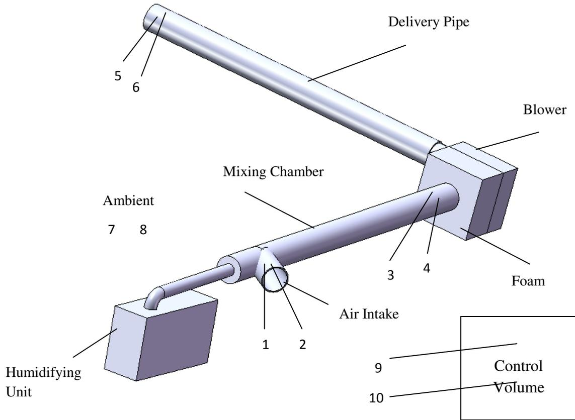
The numbers 1 through 6 signify the positions of thermocouples which were used to measure  $T_{dry}$  (odd) and  $T_{wet}$  (even) throughout the experiments.
