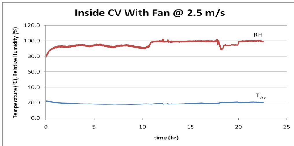
Figure 11 –  $T_{\text{dry,ambient}}$  vs. time for unit inside control volume\*
