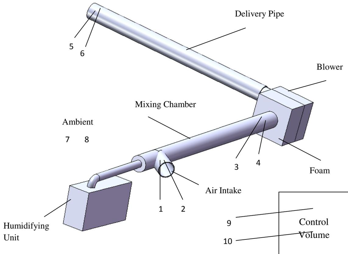
The numbers 1 through 6 signify the positions of thermocouples which were used to measure  $T_{\text{dry}}$  (odd) and  $T_{\text{wet}}$  (even) throughout the experiments.
