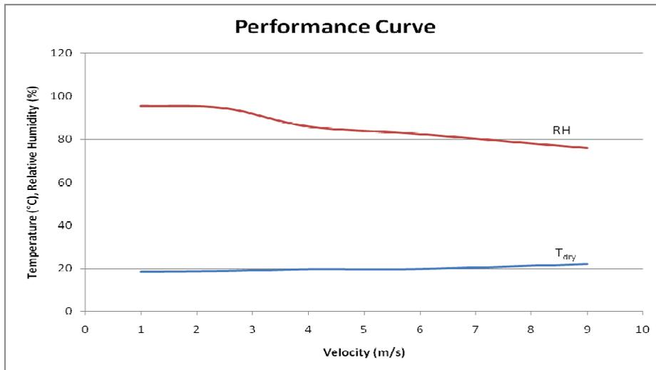
At a velocity of 4.5 m/s, the relative humidity was roughly 80%.
